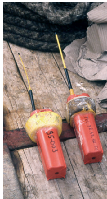
Left: surface drift buoys: independent, floating Argos beacons which can be dropped from aircraft
