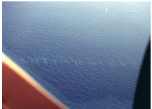
The wind slices the slicks into windrows. If the wind is strong, iridescences may disappear.
